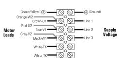
2. All leads are color coded as well as identified with a band containing an Alpha/Alpha or Alpha/Numeric code (i.e. TK or Z2). Colors should be verified against code band. If code band and color do not correspond to schematics above, wire according to the code on the band.
